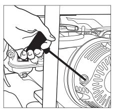
**Step 7** Pull the starter handle. If the engine fails to start after 3 pulls squeeze the trigger gun to release pressure, and repeat step 7.
